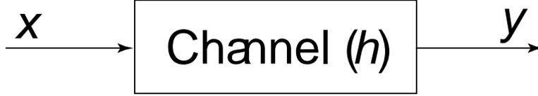
Figure 1: A single-input-single-output channel
