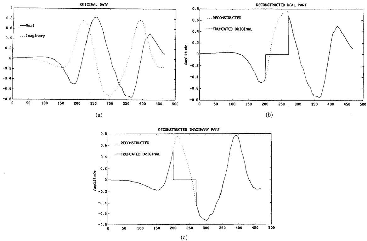
Fig. 3. These are plots of the frequency domain data of another microstrip filter [Interpolation of a considerably large number of missing points]. (a) Plot of the real and imaginary parts of the original data. (b) Plot of reconstructed real part and the original real part showing the missing points. (c) Plot of reconstructed imaginary part of the original imaginary part showing the missing points.
