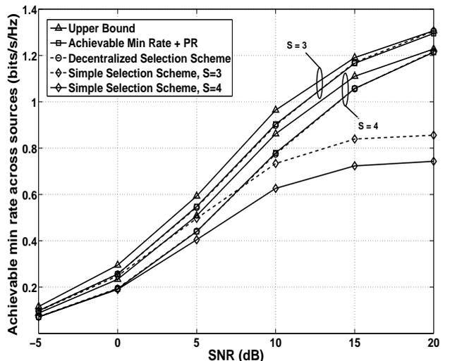
Fig. 3. Max-min rate across all source nodes of different resource allocation strategies in “i.i.d Channel” scenario with  $J = 2$ .
