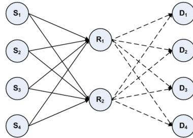
Fig. 1. Two-Hop multi-source multi-destination mesh network
