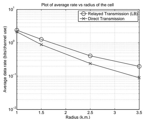
Fig. 4. Average user-rate as a function of the radius of the cell
