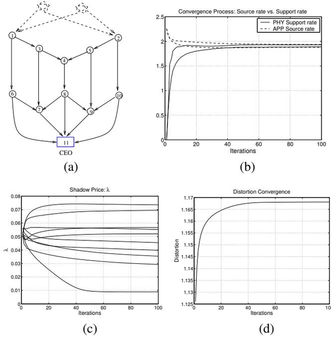
Fig. 3. (a) Sensor network topology; (b) Convergence process between source rates and capacity support, (c) Convergence process of dual variable  $\lambda$ , (d) Convergence process of network utility, i.e., estimation distortion.
