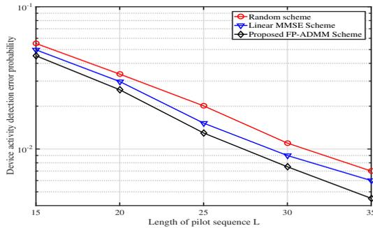
Fig. 4. Device activity detection error probability versus the length of the pilot sequences
