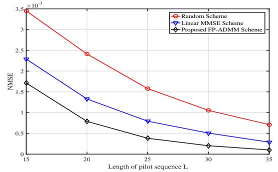
Fig. 2. NMSE performance versus the length of pilot sequence  $L$ .
