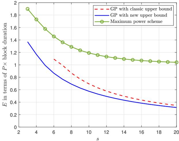
Fig. 3. Energy  $E$  vs. pathloss-to-noise ratio  $s$  when  $L = 3$  and  $\delta = 2$ .
