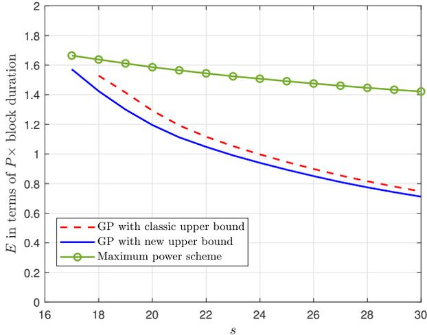
Fig. 2. Energy  $E$  vs. pathloss-to-noise ratio  $s$  when  $L = 1$  and  $\delta = 3$ .
