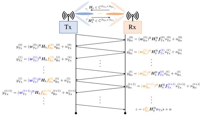
Fig. 1: Beam alignment using ping-pong pilot protocol. The sensing beamformers designed at Tx and Rx are highlighted as blue and orange, respectively. The initial sensing beamformers are fixed, hence not colored.
