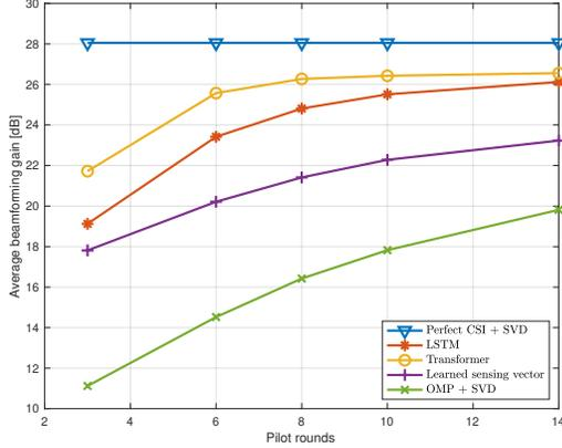
Fig. 3: Beamforming gain vs. pilot rounds,  $K = 25$ ,  $N_{Tx} = 64$ ,  $N_{Rx} = 32$ .
