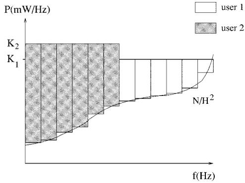
Fig. 4. A typical two-band frequency assignment.
