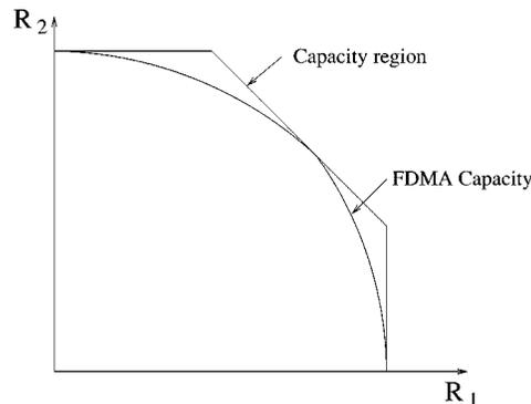
Fig. 1. The Shannon capacity region and the FDMA-capacity region of a multiple-access channel.
