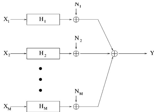
Fig. 2. A multiple-access channel.
