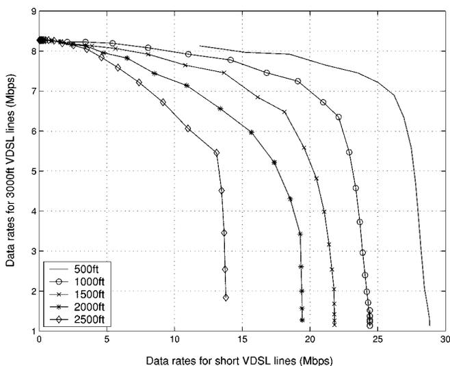
Fig. 9. Competitive optimal upstream rate regions in VDSL: 3000 versus various lengths.
