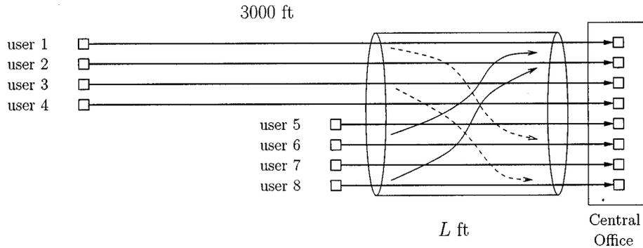
Fig. 7. Loop topology for VDSL upstream power backoff. ( $L = 500\text{--}2500$  ft.)
