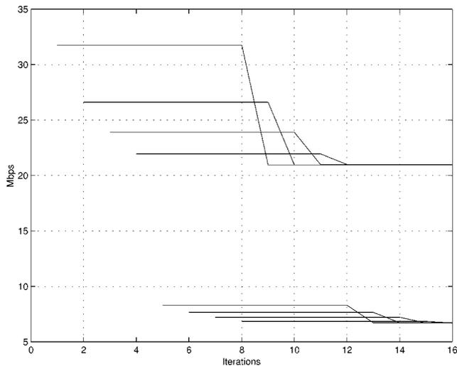
Fig. 8. Convergence of iterative water-filling algorithm. The upper four lines correspond to four 1000-ft loops at  $-15.5$  dBm. The lower four lines correspond to four 3000-ft loops at  $11.5$  dBm.
