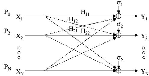
Fig. 2. A Gaussian interference network.
