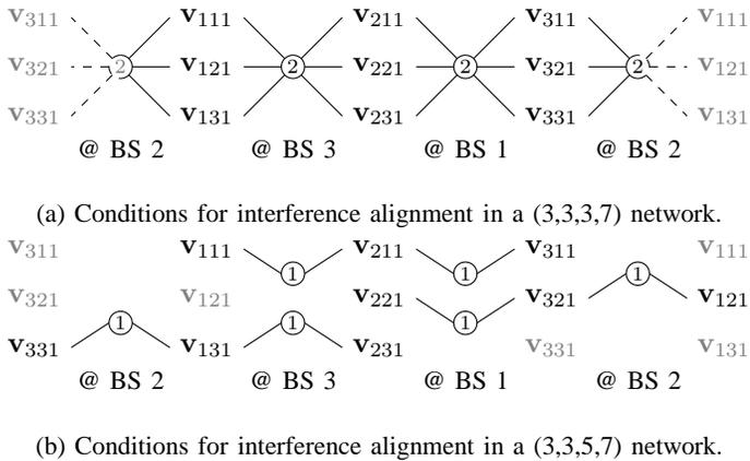
Fig. 2: Conditions for IA to achieve 1 DoF/user in two three-cell networks with three users/cell.
