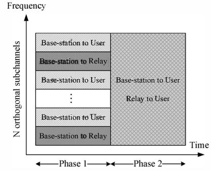
Fig. 3. Half-duplex two-phase relay frame structure
