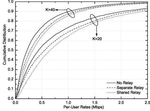
Fig. 4. Comparison of separate relay and shared relay, with  $P_r = \frac{1}{3}P_s$ .
