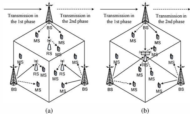
Fig. 1. Relay scenarios. (a) Separate relaying. (b) Shared relaying.
