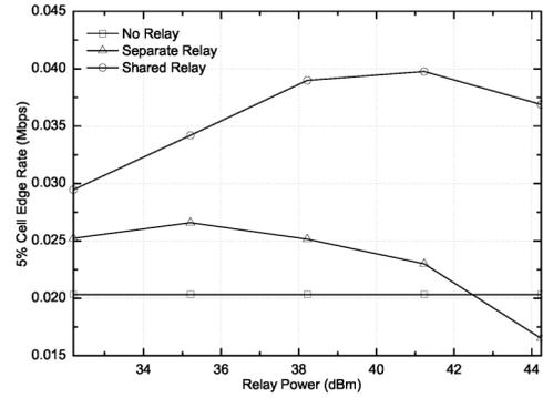
Fig. 6. Per-sector 5% cell edge rate as a function of  $P_r$  with  $K = 40$
