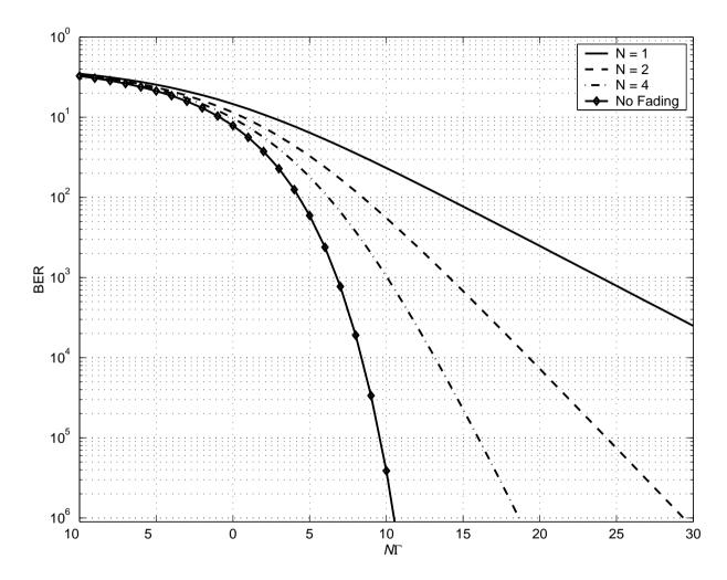
BER versus output SNR. Note that even though output SNR is the same, the BER is significantly different.
