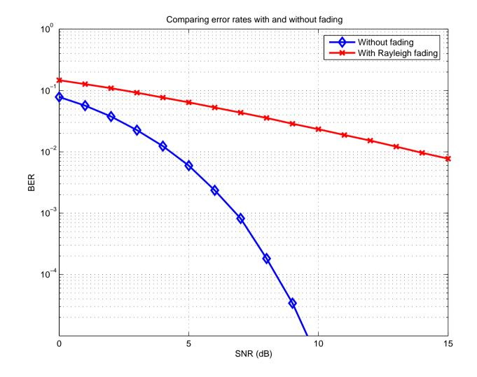
Note: In the case with fading, the BER v/s SNR plot (in log-log format appears as a straight line)
