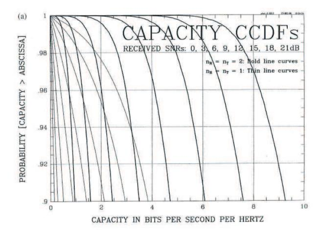
Note: "Success" rates (probability that capacity is above target) from Foschini and Gans (1998). Comparing "success" rates for SISO and a N=M=2 system.
