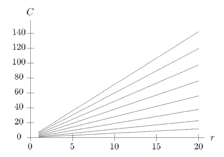
Note: Ergodic capacity for fixed SNR (from Telatar (1999)). Here r is the number of elements in the transmitter and receiver (r = M = N)
